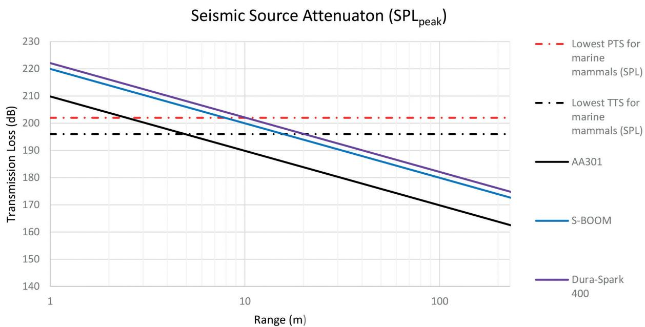
*Figure 4: Sound Pressure Level ( $SPL_{peak}$ ) attenuation based on equation Figure 2*
