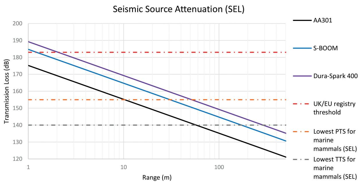
*Figure 3: Sound Exposure Level (SEL) attenuation based on equation Figure 2*
